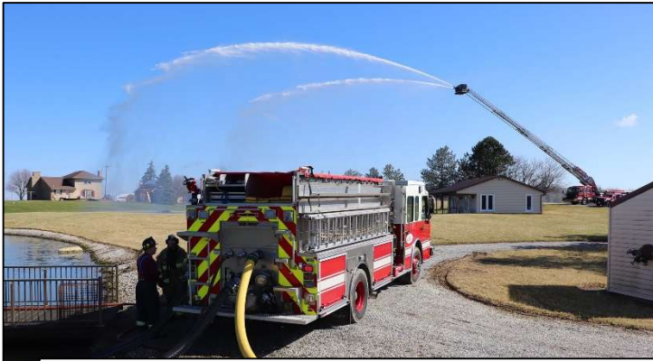
Lockington Engine 763 drafts water from the pond, the fire pump building is visible to the right. Sidney's Quint 3, at the business end of the water shuttle, sends the water back to the pond after a short but frenzied trip down the road.
