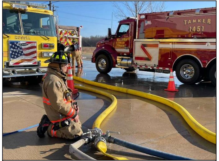
Russia’s engine crew utilized manifolds supplied from the pumper to the loading stations. These offered the crew the option of filling with a single 4” storz connection, dual 65mm storz connections, or even in some cases a combination of 4” and 65mm as time and resources allowed.
